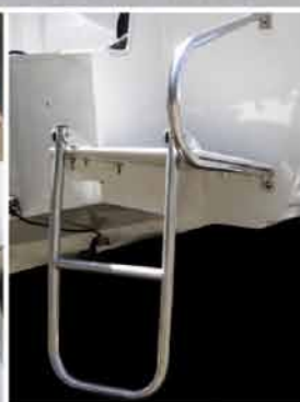
The boarding ladder makes it easy to get in and out of the water.
