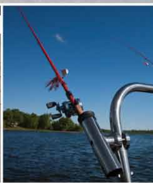
A pair of SS rod holders on the ski tow bar add convenience to angling off the stern.
