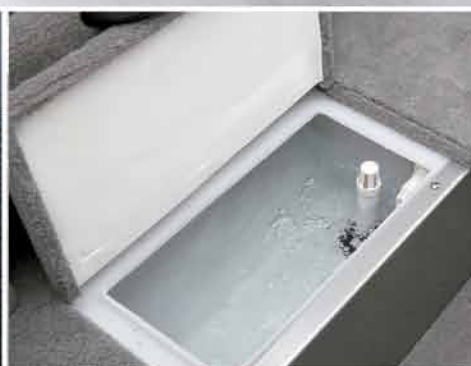
An aerated baitwell is located at the stern starboard. (1700 only; dry storage box on 1600 model)
