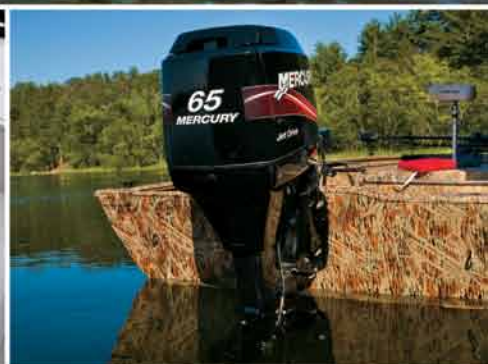
Extra-tall 27" transom designed for mounting jet engines.
