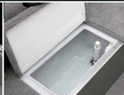
An aerated baitwell is located in the stern on the starboard side.
