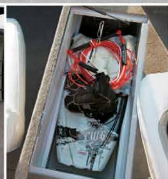
An in-floor storage compartment measures 86"x18"x11" to hold wakeboards and ropes or fishing rods and gear.
