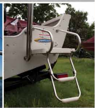
Boarding the 1800 Super Hawk is simple with the optional swim platform and ladder. (Standard on SST).
