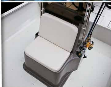
Center-mounted seat with built-in ice box/dry storage and rod holders. (Center console models)
