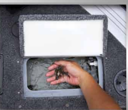
The aerated bow baitwell is elevated off the casting platform, making it easier and more convenient to access.
