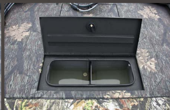
■ Aft Livewell: An aerated aft livewell (16: 22-gal.; 18: 30-gal.) includes a convenient removable divider to separate the catch.
