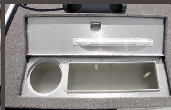
■ Aerated Livewell: Features 22-gal. capacity and a dedicated spot for a removable bait bucket.
