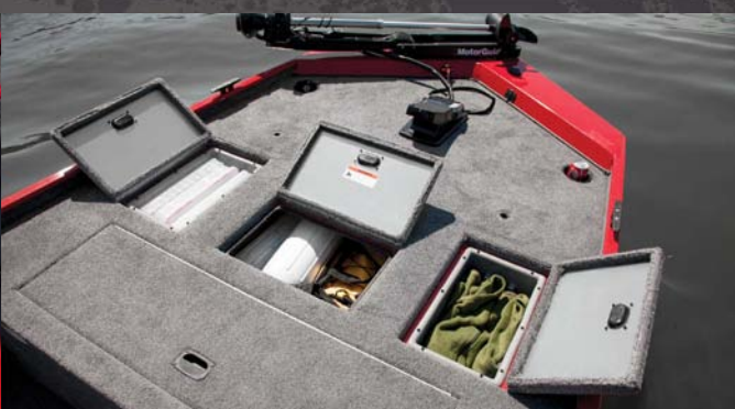
■ Bow Storage (17): Flat bow deck includes a large center storage compartment and two tackle storage bins.
