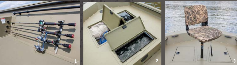
1: Starboard rod storage accommodates three rods. 2: An 18-gal. livewell and two in-floor storage compartments in bow. 3: Bow pedestal seat base standard.
