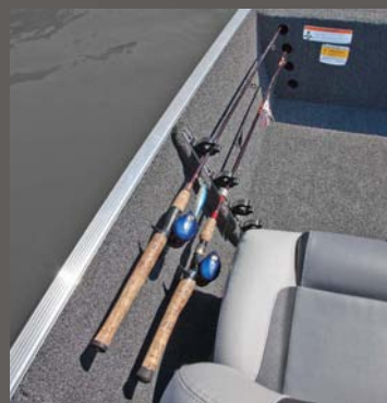
■ Port Rod Storage (16): Space-saving rack secures four rods up to 8' in length.
