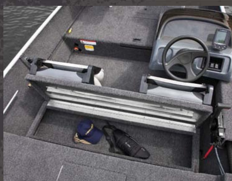
■ Under-seat Storage: The panel beneath the driver and passenger cockpit seats lifts to reveal a spacious and fully carpeted storage compartment below.
