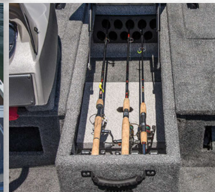
Center rod locker with reel pockets holds five 7' and five 6'9" rods.
