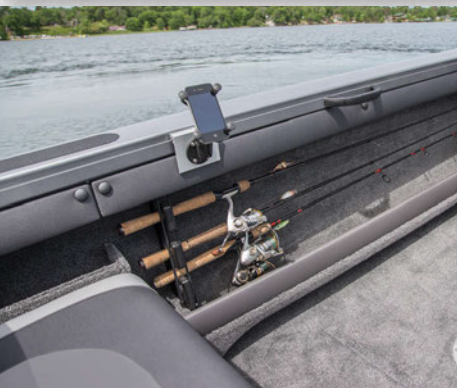
Open port storage (three tubes accommodate 8' rods) w/ convenient aft storage cubby.
