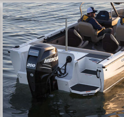
SST water-entry system: cut-away step, non-skid swim platform and under-mount ladder.
