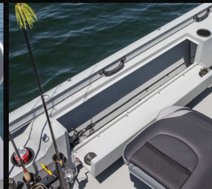
Lockable port rod storage and optional vertical rod holders
