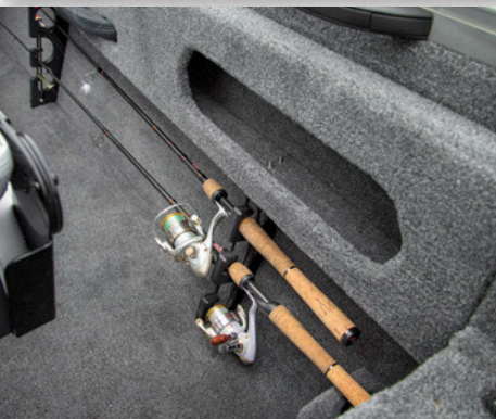
Starboard under-gunnel storage and quick-access rod rack system.
