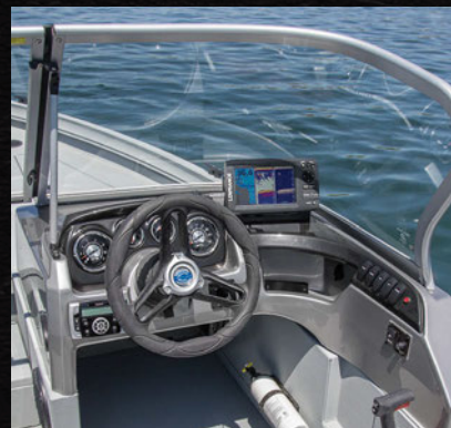
All-new fiberglass, reinforced console features hydraulic steering.
