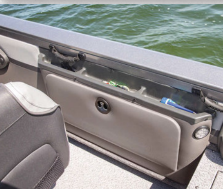
Under-gunnel starboard storage w/ door and topside quick-access trays.
