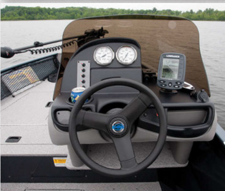
Ergonomic helm w/ curved windscreen, toggle switches and optional analog gauges.
