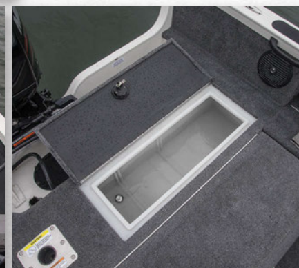
Stern 19-gal. aerated livewell. Recirculating system standard on I850, optional on I750.
